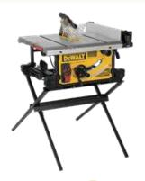
Dewalt DWE7490X Portable Job Site Table Saw With Scissor Stand, 3-1/8 in at 90 deg/2-1/4 in at 45 deg, 15 A, 120 VAC
